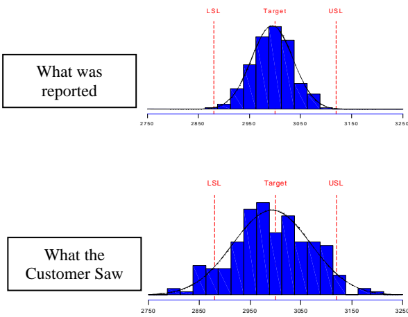
Figure 7. The problem with averages – what is reported is not what the downstream processes see.
