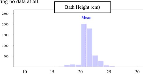
Figure 8. Manually collected bath height (cm) data. Action is required if the bath height is less than 20cm
