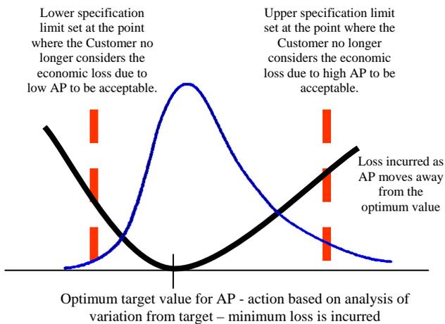
Figure 3. "On target with minimum variation" approach to control of anode core Air Permeability reduces variation and loss (new loss function)
