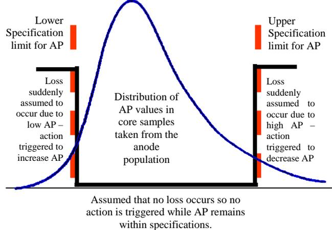
Figure 2. “Binary” control of anode core Air Permeability.
