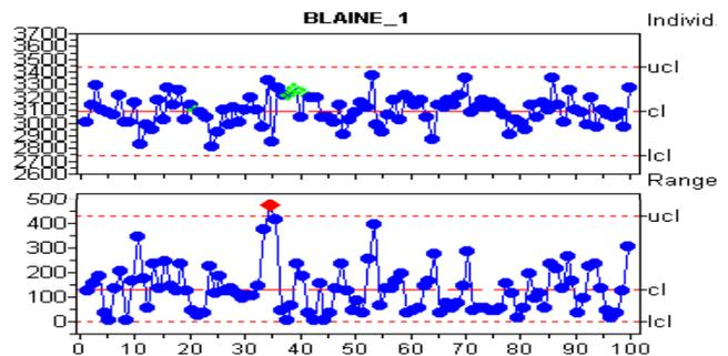
Figure 9. IMR Control chart of Blaine Index values of the fine product from Ball Mill 1 over a week.
