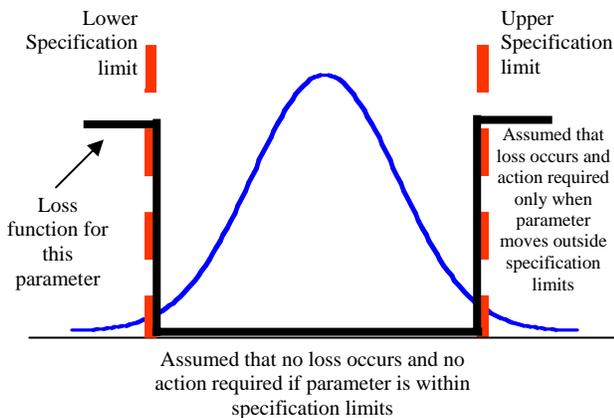
Figure 1. “Binary” control model assumes that as long as a parameter remains within arbitrary specifications no loss is incurred by the process. (See loss function curve) resulting in increased process variation and cost.
