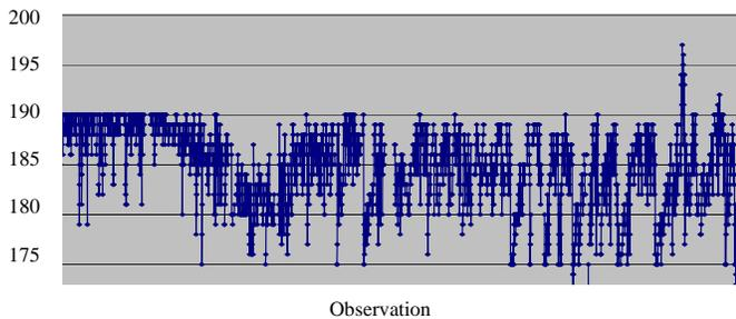
Figure 7. Manually collected mixing temperature (°C) data. Action is triggered if the reported temperature exceeds 190°C.
