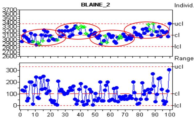
Figure 10. IMR Control chart of BI values of the fine product from Ball Mill 2 over a week. An unstable pattern of steps is evident in the data.
