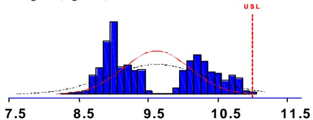
Figure 6. Histogram of individual railcar analyses of green coke VM delivered to a calciner. The average VM reported for this batch of green coke was 9.6%.
