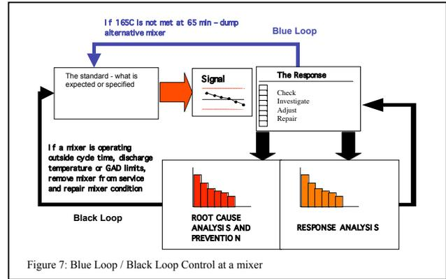
Figure 7: Blue Loop / Black Loop Control at a mixer
